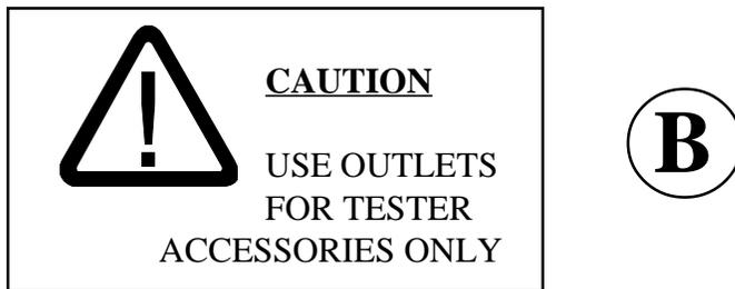
This label means that the outlets on the rear of the tester are for the tester accessories only and should not be used for miscellaneous shop tools or appliances.
